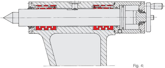
Sleeve guide in a tailstock. Minimal guide play can be achieved here during the assembly process. Guide play readjustment is possible at any time. Grease lubrication with facility for occasional re-lubrication is sufficient here.
