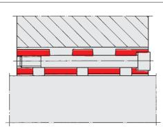
Connection with assembling play between the housing, guide bushing and centre sleeve.
