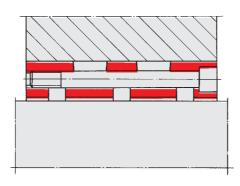
First phase of axial pre-stress: Assembling play between housing and guide bushing eliminated, firm fit realized.
