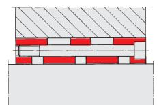
After further axial pre-stressing, the guide play between the guide bushing and sleeve is optimum adjusted.
