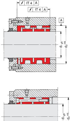
Fig. 1: Configuration of connecting components when using a series FDK or FDL guide bushing.
