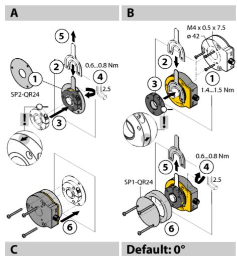
Extensive range of mounting accessories for easy adaptation to many different shaft diameters. Based on the functional principle of RLC coupling, the sensor operates absolutely wear-free and is immune to magnetized metal splinters and other interference fields. Wrong installation is hardly possible.
