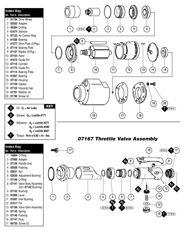
Note: On Models 14302, 14303, and 14306 the 07167 Throttle Valve Assembly can be mounted on either side of the tool for right or left hand comfort.
