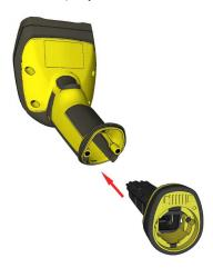
2. With a 2.5 mm Allen wrench, tighten the screws so that the slide-in is firmly locked.
