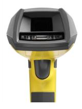
The DataMan 8050 readers offer the industry's most advanced technology for reading 1D and 2D codes regardless of size, quality, printing method or surface, and belong to the only industrial handheld ID reader family that offers Industrial Ethernet communication. DataMan 8050 is available with patented 1DMax+ with Hotbars, class-leading 2-D algorithms and future-proof modular communication slide-ins.
