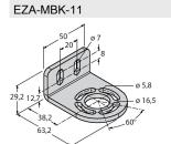
3071470 Mounting bracket, steel, blackfinished, for EZ-ARRAY and EZ-SCREEN standard and cascade 14 & 30 mm
