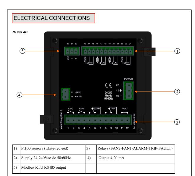
Note: relay contact image in non-alarm condition, with the exception of the FAULT relay that opens: contacts 11-12 open (NO) contacts 11-12 closed (NC) fault condition identification. Read the Alarms and Ventilation paragraph on page 13 and see the opening of the fault contact.
