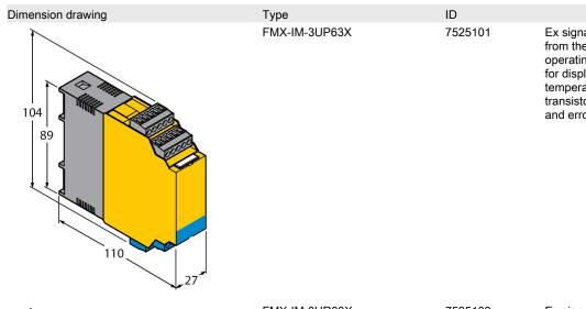
Ex signal processor for Ex flow sensors from the FC...-NAEX... family; operating voltage 20...30 VDC; LED bar for displaying flow speed and medium temperature; IO-Link device with transistor outputs for flow, temperature and errors
