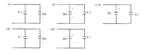
0.1uf is ceramic the other is tantalum. Noise bandwidth is from DC to 20MHz
