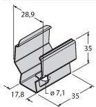
Snap bracket for mounting WLS28 work lights
