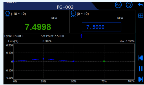
Pressure gauge / transmitter / switch calibration
