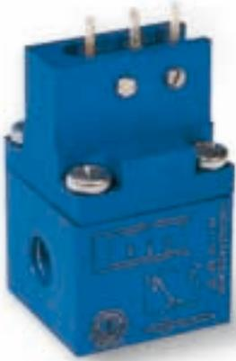
These vacuum switches feature reduced overall dimensions and give an electric signal when a certain adjustable vacuum level is reached. The pressure differential existing between the set maximum value and the value of reset of the rest signal is  $50 \div 60$  mbar and it is not adjustable.
